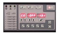
Control panel features include a programmable sequential zone start-up, seven-day programmable clock, automatic temperature setback, two user selectable inputs and one selectable output, and password protection for setup configuration
