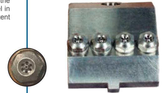
The main advantage that we provide is that we have inserts with 6 air orifices per adhesive stream for a higher frequency on the swirl, which allows customers benefit from a higher bonding as the number of crossing points of the swirl pattern increases. This feature also allows the end users to run the machine at higher speeds.
